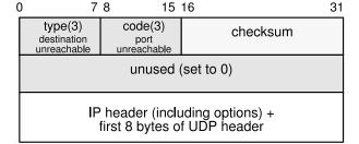
Figure 5: The diagram shows the structure of an ICMP port unreachable message. Honeyd introduces errors into the quoted IP header to match the behavior of network stacks.
