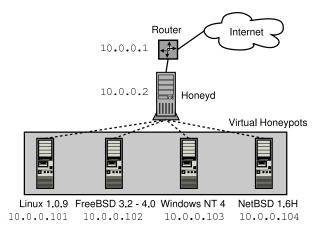
Figure 1: Honeyd receives traffic for its virtual honeypots via a router or Proxy ARP. For each honeypot, Honeyd can simulate the network stack behavior of a different operating system.
