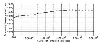
Figure 9: The graph shows the per-packet processing time depending on the number of virtual honeypots. For one thousand randomly chosen destination addresses, the processing time is about  $0.022~\mathrm{ms}$  per packet. For 250,000 destination addresses, it increases to about  $0.032~\mathrm{ms}$ .
