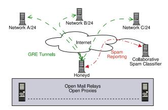
Figure 12: Using the Honeyd framework, it is possible to instrument networks to automatically capture spam and submit it to collaborative filtering systems.
