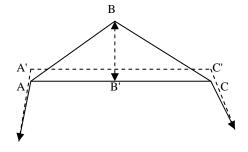
Fig. 5. Path fitting. After removing vertex B, A and C are shifted 1/4 the distance from B' to B to reduce the induced error.
