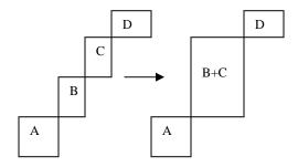
Fig. 2. Merging boxes B and C in the MBR algorithm.
