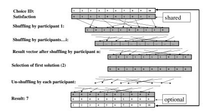
Figure 1: MPC-DisCSP4 using mix-nets
