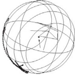
Fig. 11. Estimating the center of rotation of a marker around a segment determined by several
